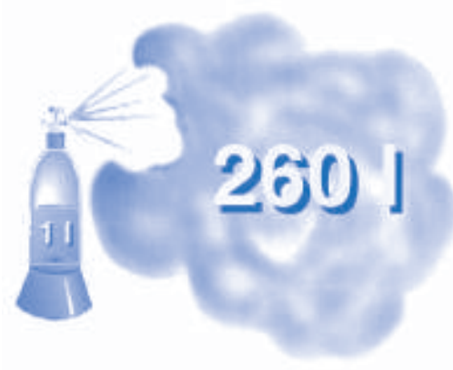
Figure 2.4. Evaporation of even small quantities of flammable liquids (such as liquefied propane) may give rise to large quantities of flammable vapours
