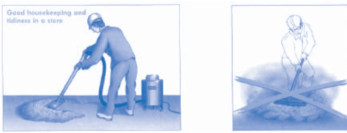
Figure 3.2. Removal of dust deposits (9)
